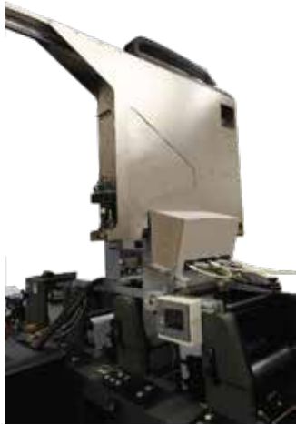
DICEblade 1 Color mounted on a flexo press
